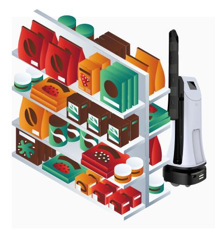
As the robot moves, it collects data and information from each tag. Our robot is able to locate itself inside a store or warehouse continuously.
