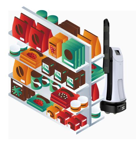
As the robot moves, it collects data and information from each tag. Our robot is able to locate itself inside a store or warehouse continuously.
